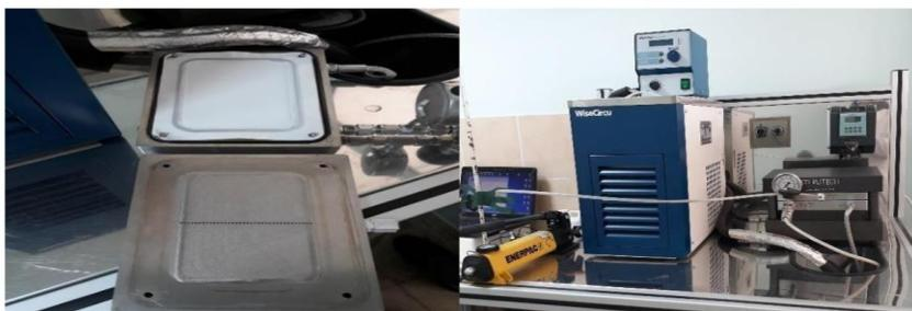
Figure 2: Cross Flow Membrane Filtration System
