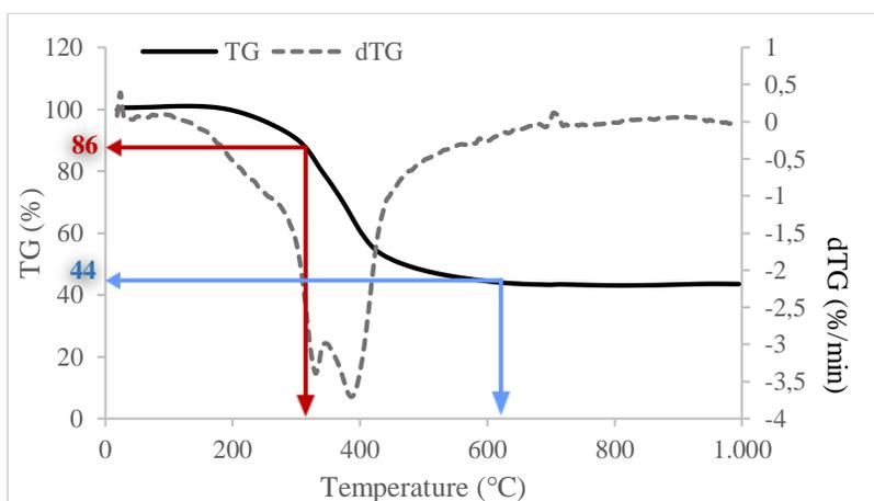
**Figure 6.** TG and dTG Curves of *PS-P50-250°C-24h*
