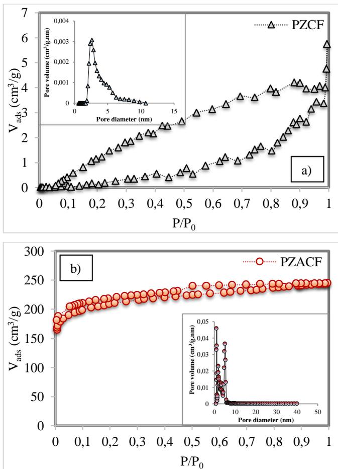
**Figure 9.** Nitrogen Sorption Isotherms and Pore Size Distribution Plots of a) *PZCF* and b) *PZACF*
